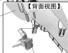
车辆线束上的夹扣 拆开 (Clasp on vehicle wiring harness, pry open)
